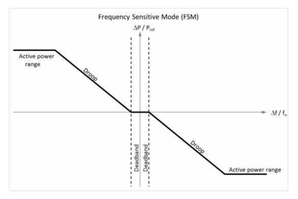
Figure 3.5: Frequency Sensitive Mode (FSM)
